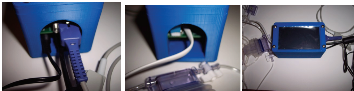
Figure 23. Photos of the connections through holes in the box (left and center) and the completed device (right).
