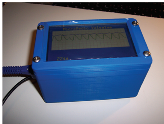
Figure 1. Photo of the prototype VTD during initial testing of the SpO2 circuit and program.
